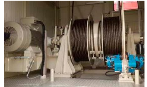
○ Boom hoist gear
